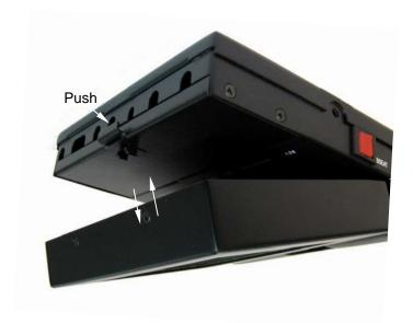
1. Push the latch to lift up to release or down to lock the LCD Monitor.
