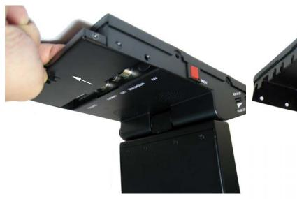
3. Slide out the wiring cover as shown above.
