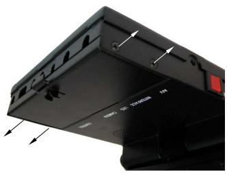
2. Remove all 4X - M3 Countersunk Phillip Head Screws using a proper screw driver.
